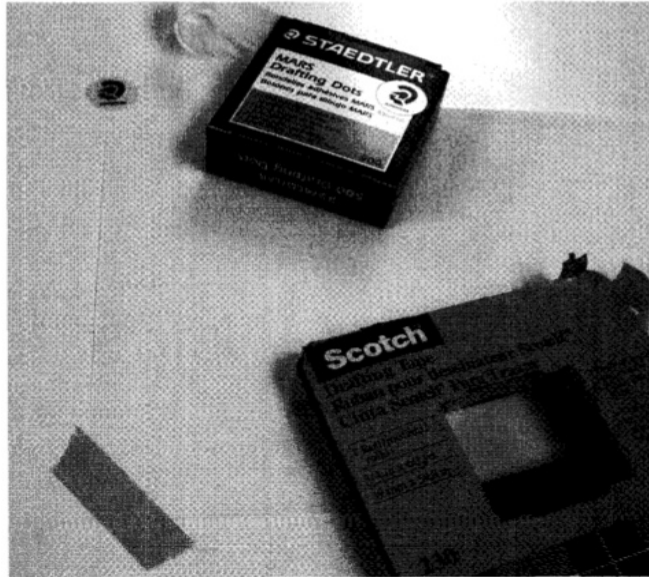
Figure 8 Drafting Dots Tape (bottom) or dots (top) used to anchor the corners of drawing.
