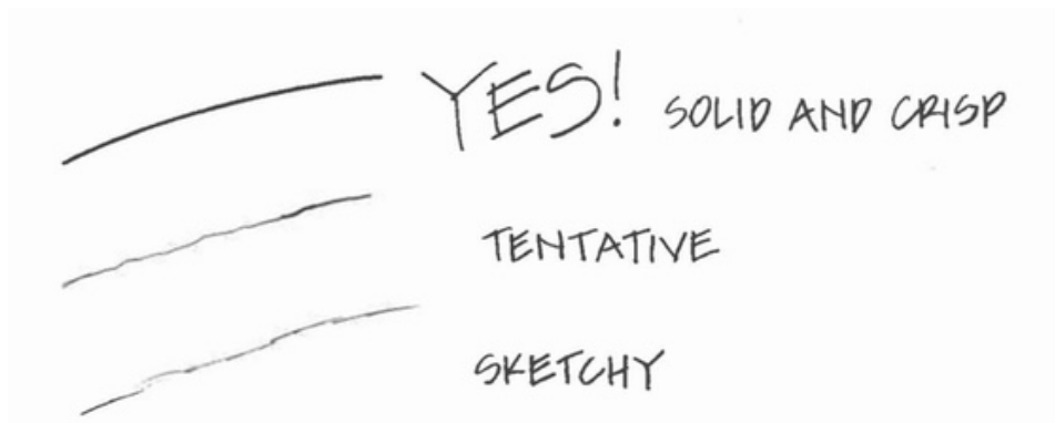
Figure 3-3 Line Quality Keep lines solid and crisp. Sketchy lines do not read well on a plan drawing.
