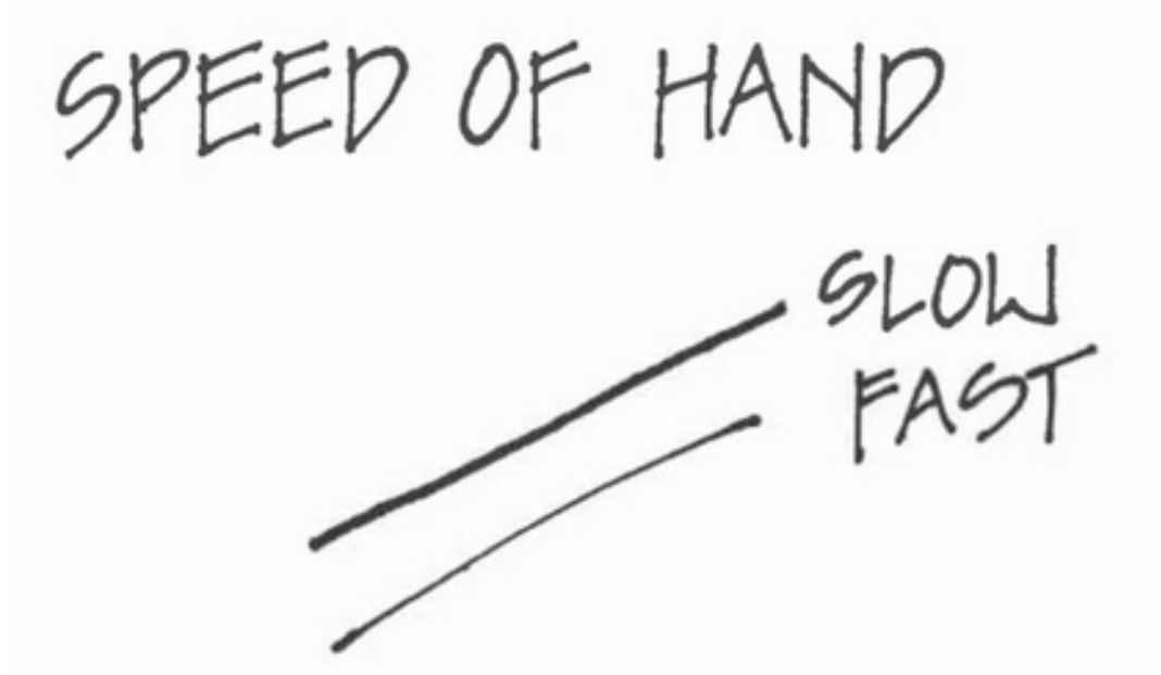
Figure 3-2 Speed of Hand As the drawing hand moves faster, the line becomes thinner and lighter.
