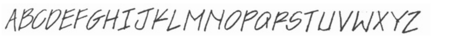
Figure 4-19 Slanting Letters Vertical axis is slanting to the right and the horizontal axis is slanting upward, or 0 degrees.
