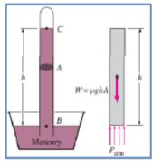
**Example 1.1:-** A manometer is used to measure the pressure in a tank. The fluid used has a specific gravity of 0.85, and the manometer column height is 55 cm, as shown in Figure. If the local atmospheric pressure is 96 kPa, determine the absolute pressure within the tank.
