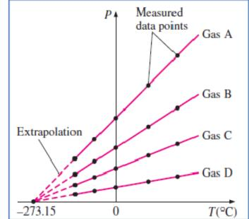
*P* versus *T* plots of the experimental data obtained from a constant-volume gas thermometer using four different gases at different (but low) pressures.
