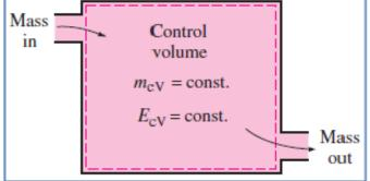
Under steady-flow conditions, the mass and energy contents of a control volume remain constant.
