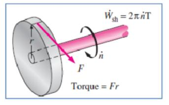
• The power transmitted through the shaft is the shaft work done per unit time, which can be expressed as  $\dot{W}_{\rm sh} = 2\pi \dot{n} T$  (kW)
