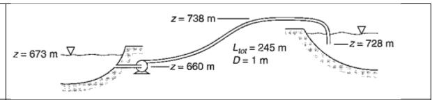
Pr.63 Water is pumped using a pump at a rate of 25 m3/s from the reservoir and out through the steel pipe, which has a diameter of 1.5 m as shown in the Figure. Assume  $\approx 1$  for all calculations in this problem. Answer Problems (4-7): Note the following: Water:  $\mu=1.31\times10^{\circ}(-3)$  kg/m.s,  $\rho=1000$  kg/m<sup>3</sup> and  $\gamma=9810$  N/m<sup>3</sup> Steel: roughness ( $\epsilon=0.046$  mm) K\_L for inlet (well-rounded) = 0.03 K\_L for exit (sharp-edged) = 1.0
