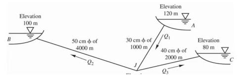
Pr.79 Three reservoirs A, B, and C are connected by the pipe system shown in the figure. If the flow rate from reservoir A is 60 liters/sec, find the height of water level in reservoir C. Determine the discharge into or from the reservoirs B and C. Take f = 0.024 for all pipes.
