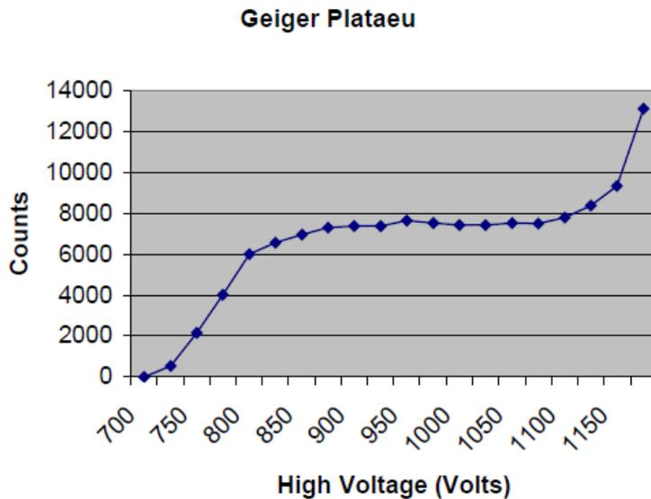
10. One way to check to see if your operating voltage is on the plateau is to find the slope of the plateau with your voltage included. If the slope for a GM plateau is less than 10% per 100 volt, then you have a “good” plateau. Determine where your plateau begins and ends, and confirm it is a good plateau.
