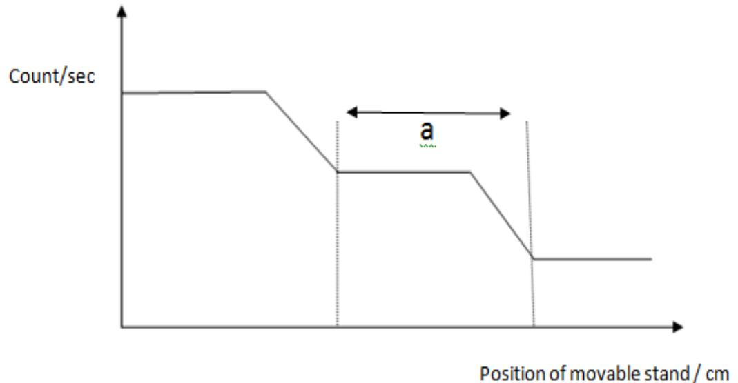
Fig (2): Gamma-quanta rate versus movable stand level.
