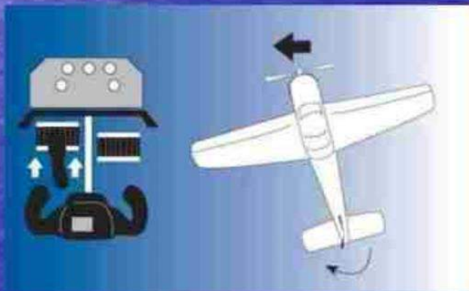
Push right rudder pedal and the plane turns right
