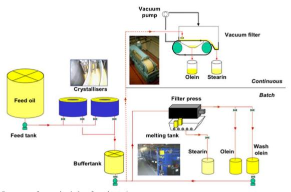
Layout of a typical dry fractionation process.
