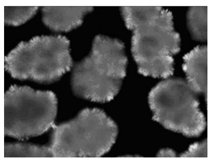
Polarized light microscopic picture of typical spherulitic crystals developing in palm oil fractions.
