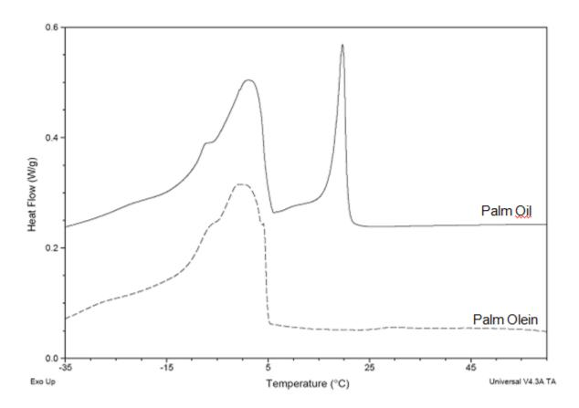
DSC cooling profile (-5°C/min) of palm oil and its derived palm olein fraction. Exothermal peaks are shown upwards.
