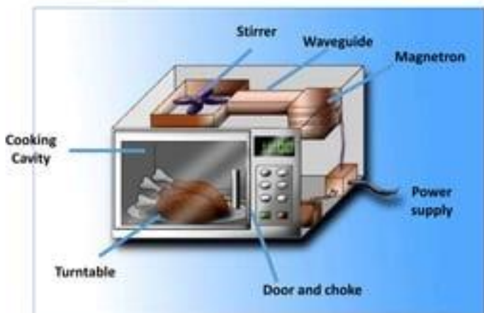
BASIC STRUCTURE OF MICROWAVE OVEN
