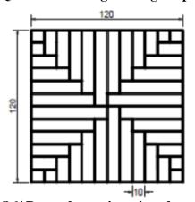
Q6/ Draw the engineering shape using the drawing instruments. (Note; scale 1:1).
