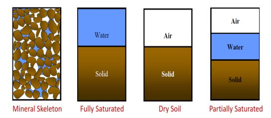
To develop the weight–volume relationships, we must separate the three phases (that is, solid, water, and air) as shown:
