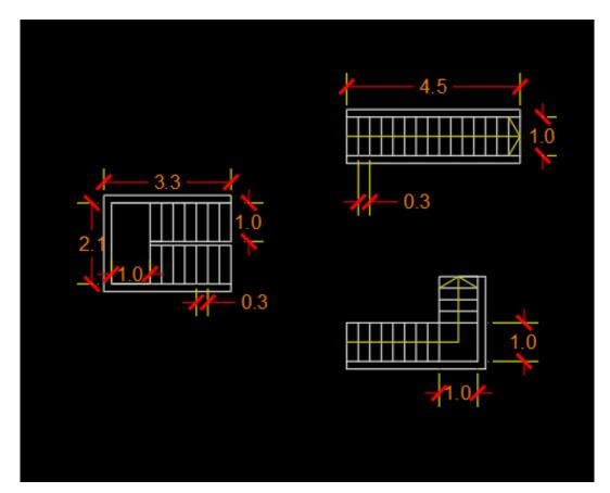
${\bf Q}{:}$  Draw the following plan as shown below using Autodesk AutoCAD programme .
