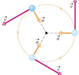
The rate of change of this angular displacement with respect to time is given by  $\vec{w} = \frac{\Delta \theta}{\Delta t}$ and this change is called "**angular velocity**". For the limit condition;  $\vec{w} = \lim_{\Delta t \to 0} \frac{\Delta \theta}{\Delta t} = \frac{d\theta}{dt} \implies \vec{w} = \dot{\theta}$ .
