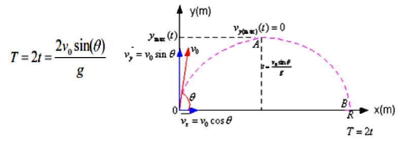
To find the maximum height  $h(y_{max})$  we use the equation  $v_y^2(t) = v_{0y}^2 - 2gy(t)$   $R = \frac{v_0^2 \sin(2\theta)}{g}$   $0 = v_{0y}^2 - 2gy(t)$ , and  $\vec{v}_{0y} = v_0 \sin(\theta)\hat{j}$ , then  $0 = (v_0 \sin^2(\theta)) - 2gy_{max}$ , finally  $y_{max} = \frac{v_0^2 \sin^2(\theta)}{2g}$ 13 **Example:** Suppose that in the example above the object had been thrown upward at an angle of 37° to the horizontal with a velocity of 10m/s. Where would it land? **Solution:**
