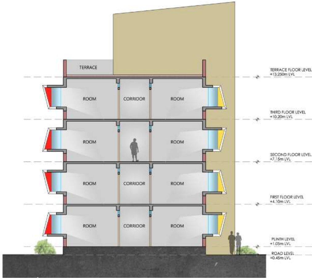
TYPICAL HOSTEL WING SECTION
