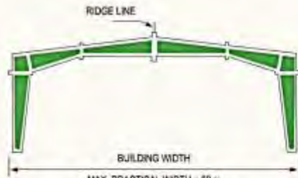
Tapered Column Clear Span (TCCS)
