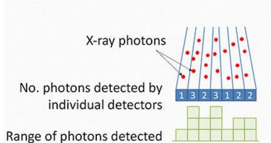
Range of photons detected shown in graph This is the dominant source of noise in an image. Photon registration by the detectors is a stochastic process. The number of photons detected will vary randomly about a mean value and that variation is the noise. The noise in the final image is given by:
