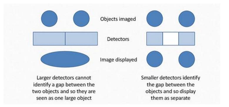
The minimum trans-axial resolution is determined by **the actual detector size**, however it is often quoted as the "**effective detector width**" at the isocenter of the scanner (Centre of the bore of the scanner). The "effective detector width" and the actual detector size are slightly different due to the divergence of the beam. The smaller the "effective detector width" the higher the resolution.
