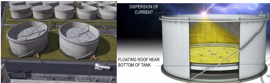
Floating roof tanks
