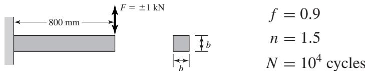
For AISI 1045 HR steel,  $S_{ut} = 570 \text{ MPa}$  and  $S_y = 310 \text{ MPa}$
