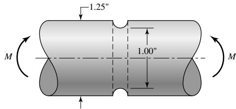
Rotation is presumed.  $M$  and  $S_{ut}$  are given as deterministic, but notice that  $\sigma$  is not; therefore, a reliability estimation can be made.
