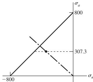
$$n_f = \frac{307.3(10^6)}{2009P} \Rightarrow P = \frac{307.3(10^6)}{3(2009)} = 51.0(10^3) \text{ N} \\ = 51.0 \text{ kN} \quad \text{Ans.}$$
