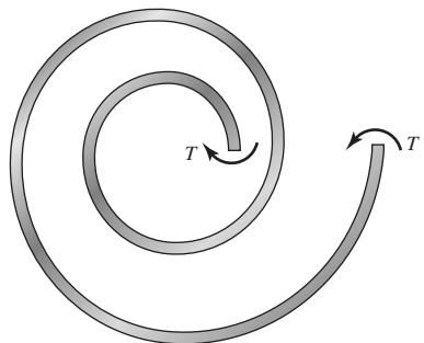
Curved beam in pure bending where  $M = -T$  throughout. The maximum stress will occur at the inner fiber where  $r_c = 20 \text{ mm}$ , but will be compressive. The maximum tensile stress will occur at the outer fiber where  $r_c = 60 \text{ mm}$ . Why?
