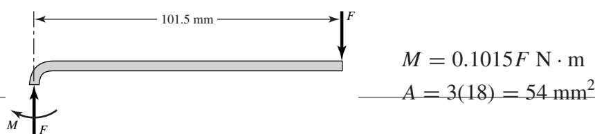
$$\text{Curved beam: } r_n = \frac{h}{\ln(r_o/r_i)} = \frac{3}{\ln(6/3)} = 4.3281 \text{ mm}$$
