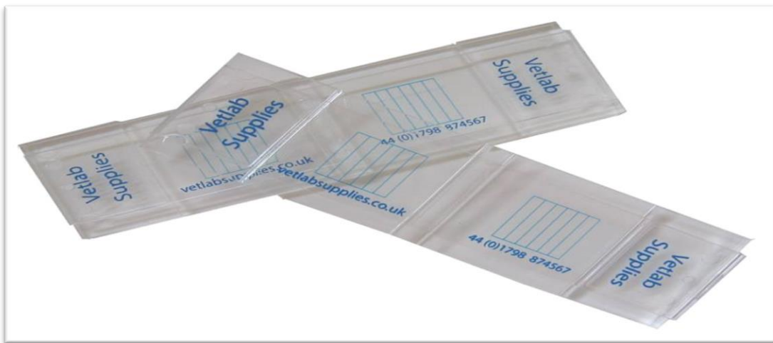
Figure 1: McMaster egg counting slide for FECRT.
