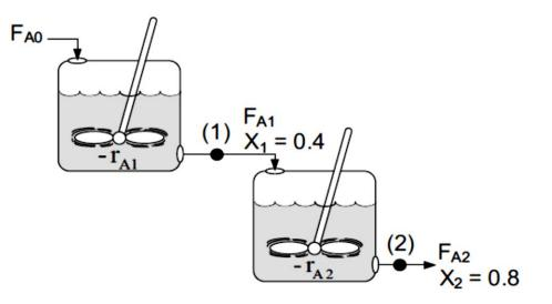
For the **first reactor**, the rate of disappearance of A is  $-r_{A1}$  at conversion  $X_1$ .
