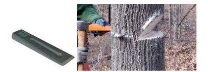
**IN FELLING:-** the wedges are inserted in the back cut to prevent the weight of the tree from closing the cut and binding the saw and also to lift and incline the tree to fall in the desired direction.
