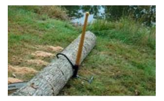
**LOG JACK**: - is a tool sometimes used when bucking trees to short lengths in some regions, particularly for pulpwood or other similar products, as the name implies, this tool is designed to jack up the tree being bucked to permit bucking without saw pinching.
