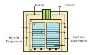
These types of dryers are useful when the production rate is small. They are used to dry wide range of materials, but have high labor requirement for loading and unloading the materials, and are expensive to operate. They find most frequent application for drying valuable products. Drying operation in case of such dryers is slow and requires several hours to complete drying of one batch. With indirect heating often the dryers may be operated under vacuum.
