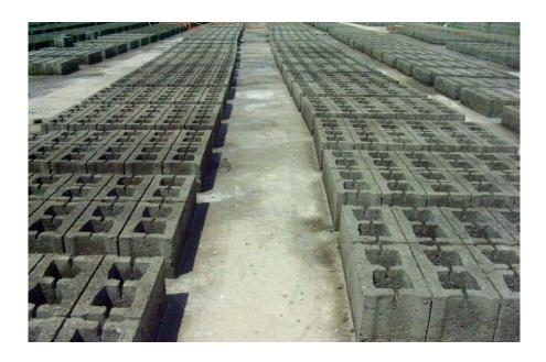
Concrete blocks are manufactured and used in three types:
