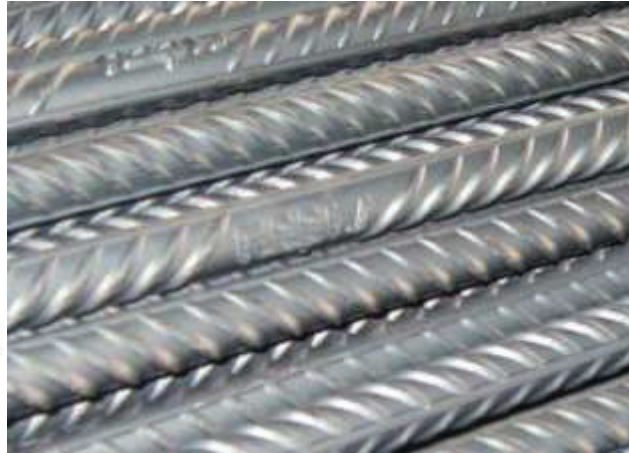
Figure 7-1.—Various types of deformed bars.
