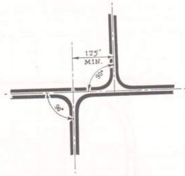
Fig. 8 More desirable street intersection.
