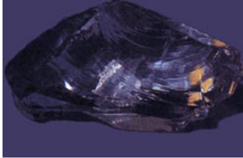
Conchoidal Fracture Quartz
