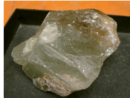
Conchoidal Fracture Quartz
