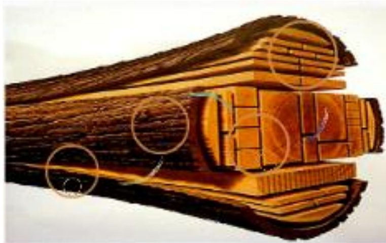
Common log sawing patterns: (a) live (plain) sawing, (b) quarter sawing, (c) combination sawing.
