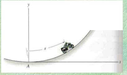
$\frac{1}{2}m\dot{s}^{2} + V(s) = E = const.$ ...Energy equation for motion of the particle on the curve Differentiating the energy equation with respect to t:  $\frac{d}{dt}\left[\frac{1}{2}m\dot{s}^{2} + V(s) = E\right] \longrightarrow m\ddot{s}\ddot{s} + \frac{dV(s)}{ds}\frac{ds}{dt} = 0$  $F_{s} = m\ddot{s} = -\frac{dV(s)}{ds}$ ...Differential equation for motion of the particle on the curve is the component of the external force in the direction of *s*
