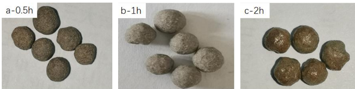
Fig.9 Effect of holding time on macroscopic morphology of ceramsite
