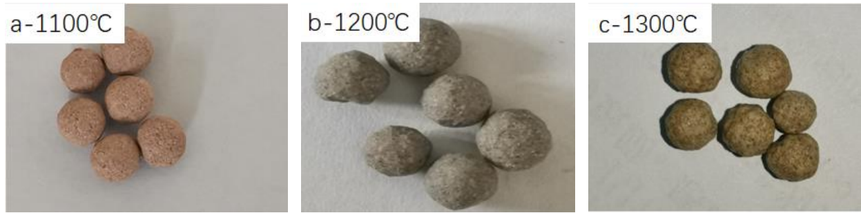
Fig.5 Effect of calcination temperature on macroscopic morphology of ceramsite
