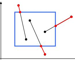
For lines with one end-point inside the window and one end-point outside, calculate the intersection point (using the equation of the line) and clip from this point out
