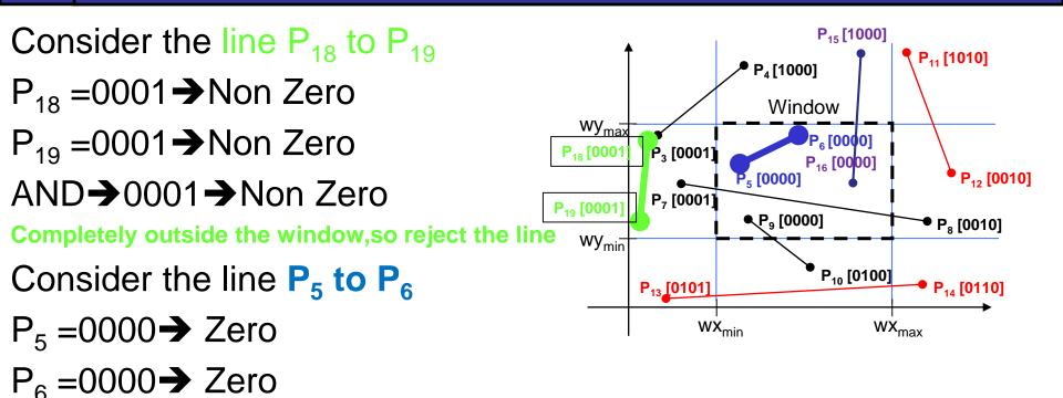
AND $\rightarrow$ 0000 $\rightarrow$ ZerO, which indicates that the line P<sub>5</sub> & P<sub>6</sub> are completely inside the window and no clipping is required, so accept the line.
