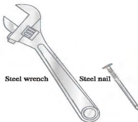
Figure [1]: Two objects with different masses and different volumes but the same density.
