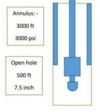
**Exercise-8**/ Calculate the mud volume required to fill the hole per stand when pulled dry if you know *Drill pipe capacity* =  $0.01776 \ bbls/ft$
