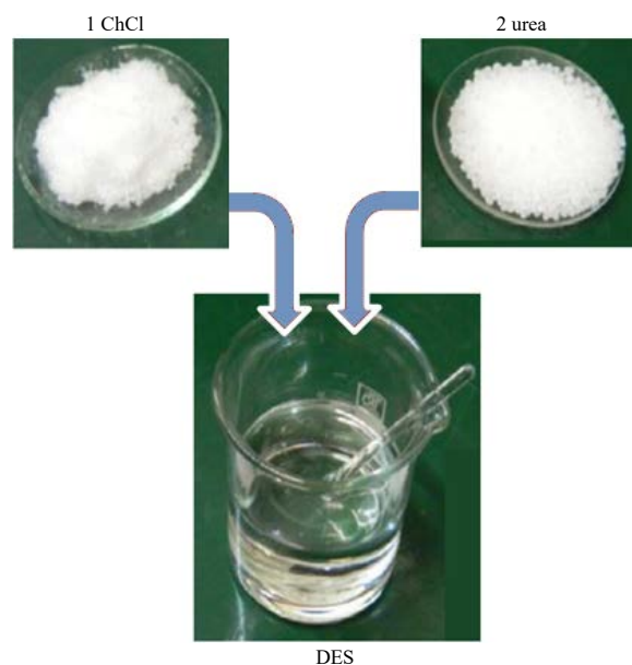
Fig. 3: Graphical representation of formation DES from 1 ChCl and 2 urea
