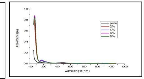
**Figure (3)**Shows the absorption coefficient of membranes (PVA) Dopedwith (COCl) with different doping ratios. **Figure (4)** Shows the energy gap values of pure (PVA) membranes .
